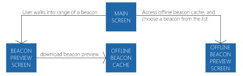
The client self was coded using the BLE API made public by RadiusNetworks [30]. This enables the application to scan for beacons once a second, and calculate their distance from the device using the RSSI that is sent with each advertisement. This distance, however, is not entirely ac-
