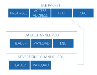
Figure 2.3: Different PDU Channel Uses
