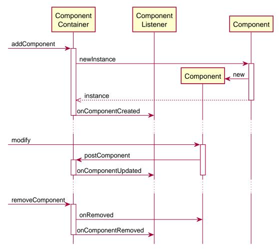
Figure 7.3: Component instance lifecycle
