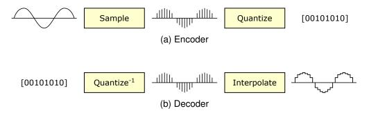
Figure 3.1: A PCM encoder and decoder [4]
