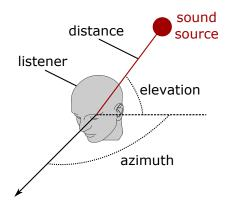
Figure 3.9: The coordinate system used for positional audio
