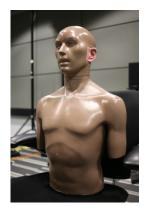
Figure 3.12: A KEMAR dummy head with pinnae [61]
