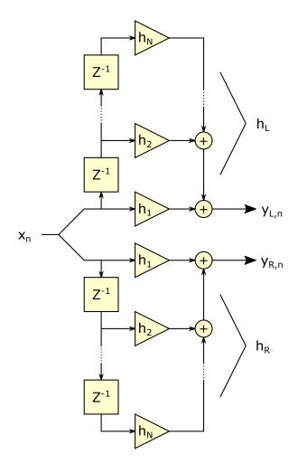
Figure 3.13: Convolution using a separate FIR filter for each ear [2]
