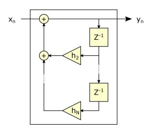
Figure 3.8: An infinite impulse response filter
