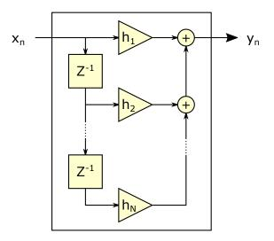
Figure 3.7: A finite impulse response filter
