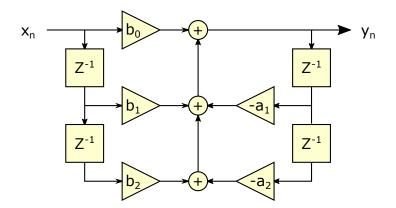
Figure 5.3: A biquad filter in direct form 1 [68]
