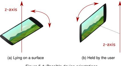
Figure 5.4: Possible device orientations
