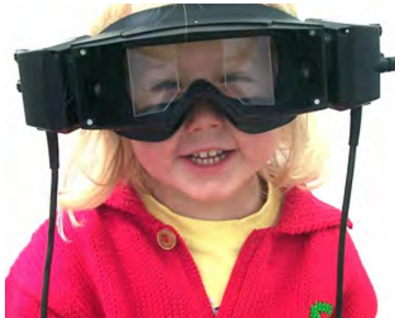
Figure 3.9: The 3D VOG Video-Oculography System by SensoMotoric Instruments is a head-mounted infrared video-oculography system for horizontal, vertical and torsional eye movements [Insa].
