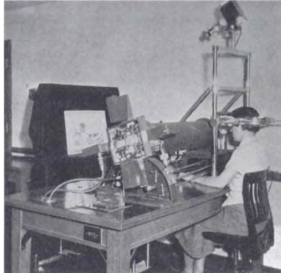
Figure 3.4: With Buswell's eye tracker, reflections from the eye's surface were recorded to measure the participant's eye movements. A series of lenses and mirrors were used. In this way the user's view was not covered [WT05].
