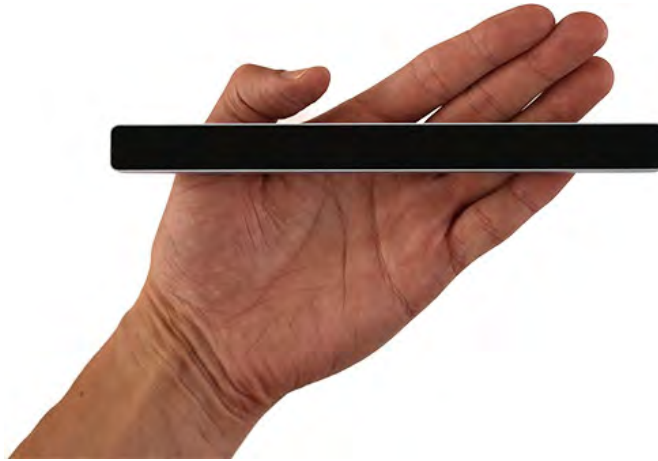
Figure 3.19: The EyeTribe tracker is a low-cost, video-based tracker. The accuracy for gaze measurement averages between 0.5 and 1.0 degrees [Eyeh].
