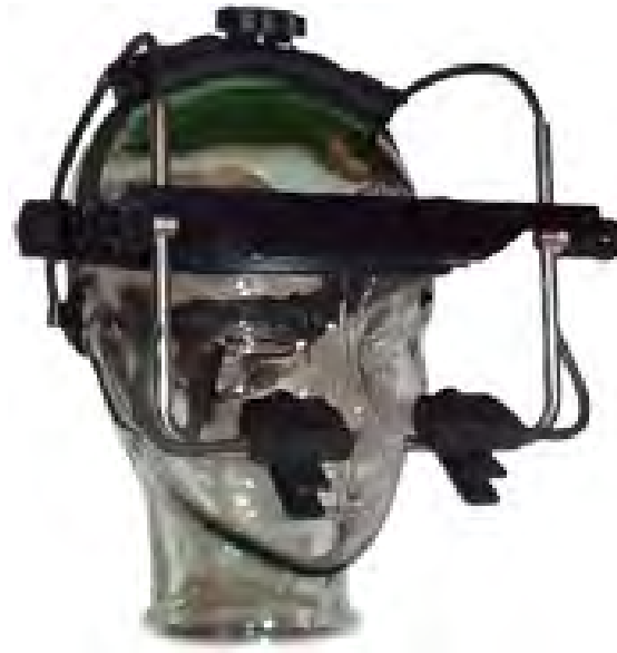
Figure 3.14: EyeLink II , introduced by SR Research, is an infrared video-based eye tracker. It works with an accuracy of 0.5 degrees [Ltd].
