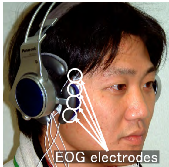
Figure 3.7: Electro-Oculography : Electrodes integrated in headphones to measure relative eye movements [MF06].
