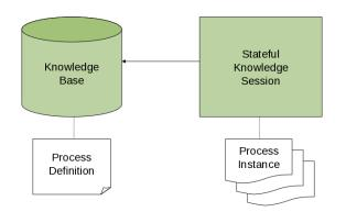
Figure 3.1: Overview of jBPM's Core Engine API [15]
