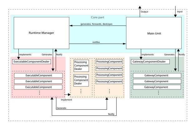
Figure 5.4: Architecture of the developed engine
