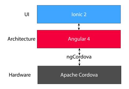
Figure 6.1: Stucture of the Ionic 2 framework
