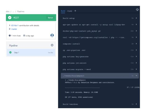
Figure A.6: Successful Bitbucket Pipeline
