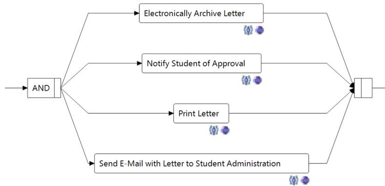
Figure 3.7: Activity Parallelization in AristaFlow
