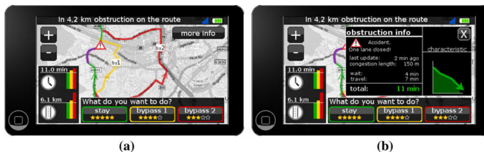
Fig. 2 Improved user interface for integrating dynamic traffic information. a Route with obstruction and alternatives, b details about traffic obstruction
