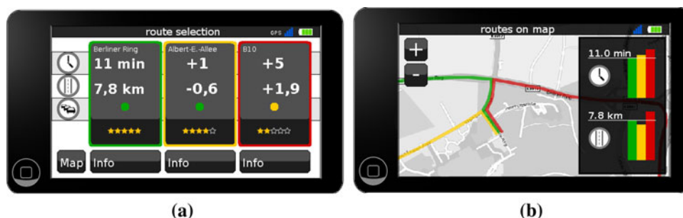
Fig. 1 Improved user interface for route selection. a Multiple routes on main screen, b multiple routes on map screen
