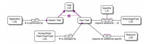
Figure 5: Multiple Resources Assignment, from [OWF<sup>+</sup>10]
