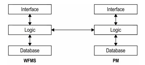
Figure 3: Integration of Workflow Management System and Project Management, from [Buss98]
