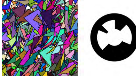
Figure 3.2: An example of other types of markers: left a feature marker, right a rotary marker.
