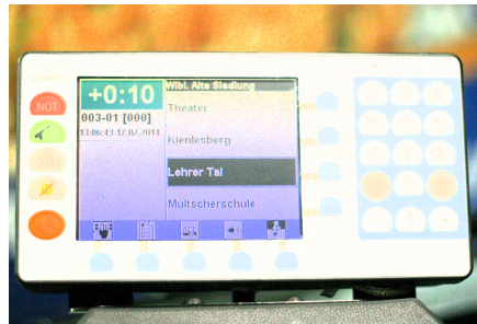
(c) The MDT user interface located within the driver's view, currently showing deviation from the scheduled departure time, and upcoming stops. At stops, guaranteed transfers can request the driver to wait for delayed vehicles.
