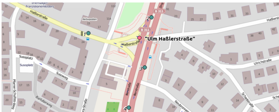
Figure 8: Geodata example of Haßlerstraße, plotted in QGIS onto map material from OpenStreetMap. The green markers are the stop point positions from the KML file, while the red marker is the stop area location as found in DIVA ’s internal exchange format and lies approximately between all four stop points. Map background © OpenStreetMap contributors [67].
