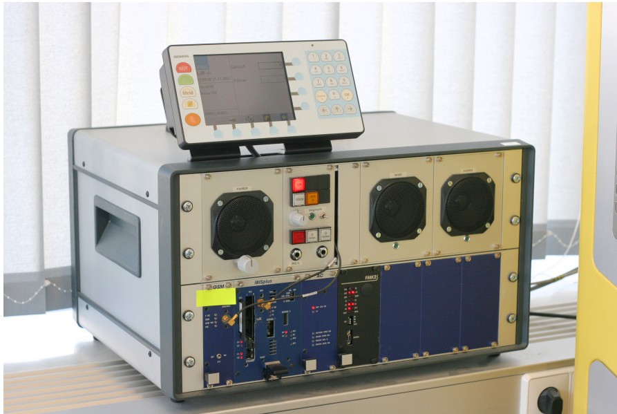
(a) Testing setup employed by SWU. The IBIS rack is at the bottom; from left to right: GSM module, IBISplus computer with connected CF storage and GPS antenna, power supply, and RF transceiver. The upper rack emulates vehicle functions, e. g., the door opening mechanism. On top sits the driver's MDT user interface.
