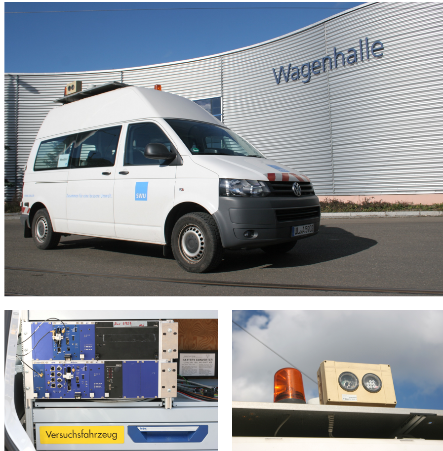
Figure 4: Test car used by SWU Verkehr. The vehicle is outfitted with two IBIS computers in the back, one in the version used for city buses, one in the version for regional buses (lower left image). In order to accurately measure positions of, and distances between stops and infrared beacons, an IR transceiver sits on the vehicle's roof (lower right image).
