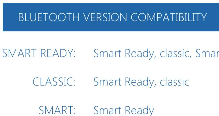
Figure 2.1: Bluetooth Version Compatibility Comparison
