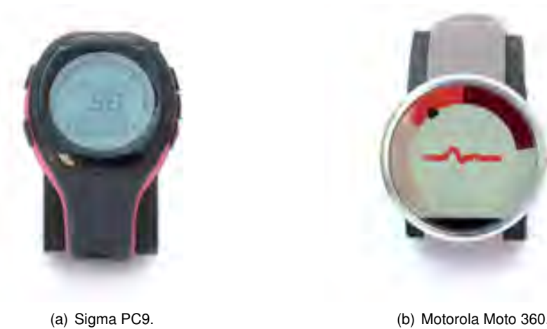
Figure 4.10: The watch component of the Sigma PC9 heart rate monitor showing a heart rate of 98 bpm (a) and the Motorola Moto 360 smartwatch showing its Moto Body Heart Rate application currently measuring (b).
