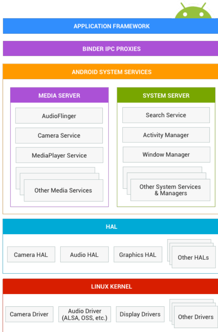
Figure 4.1: A high level view of the Android system architecture in respect of hardware support [13].
