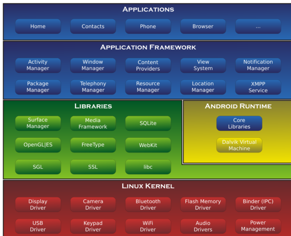
Figure 3.1: The Android architecture is composed of four main layers and five sections [40].
