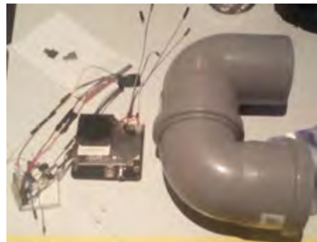
Figure 2.2: Typical self-made sensor for measuring mass concentration in the air. Image by [41] ©.
