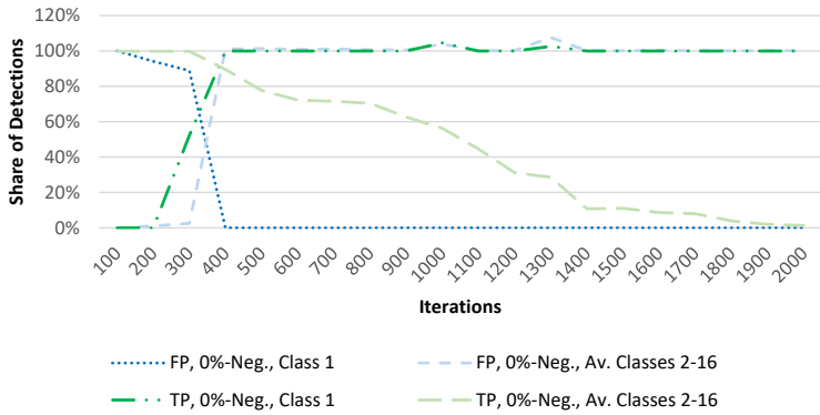
Figure 11: Re-training without negative samples (CNN_2b)
