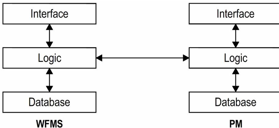
**Figure 3:** Integration of Workflow Management System and Project Management, from [Buss98]
