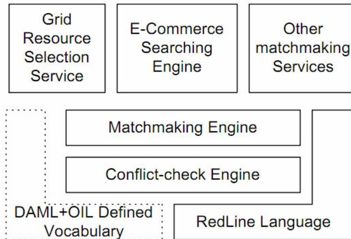
Figure 2: Redline Components, from [LiFo03]
