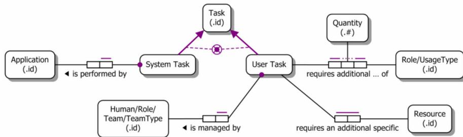
**Figure 5:** Multiple Resources Assignment, from [OWF<sup>+</sup>10]
